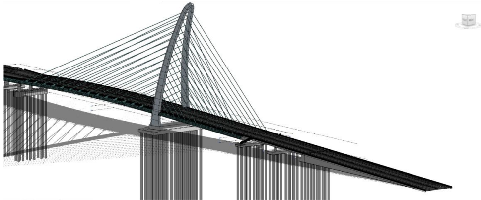
Figure 3. Modeling Thu Thiem 2 bridge with Revit 2019 at LOD 200.
