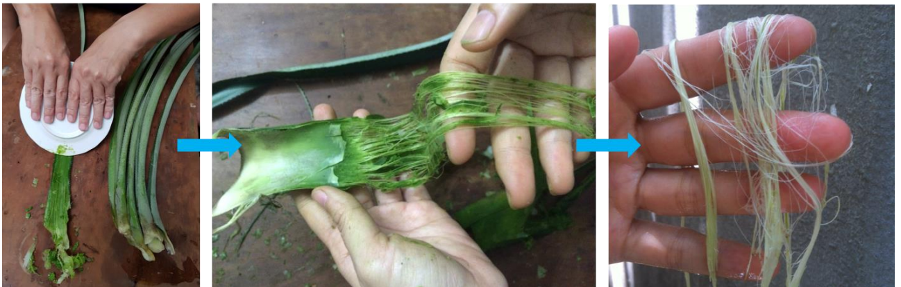
Figure 9. Preparation of fiber from pineapple leaves by manual shredding
