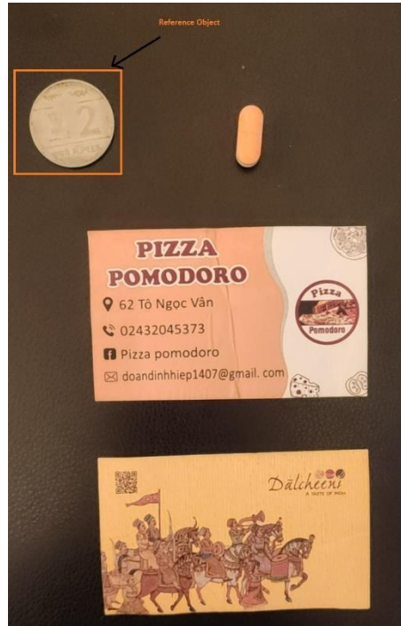
Figure 1.1. We used a two Indian national rupee coin as our reference object. By ensuring the coin is the left-most object, we are able to sort our object contours from left-to-right, grab the coin (which is able continuously be the primary contour within the sorted list), and utilize it to characterize our pixels_per_metric, which we characterize as:
