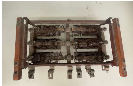
Figure 3. Dummy loader for testing paralleled MOSFETs
