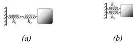
Figure 2. Serial springs (a) and parallel springs (b)
