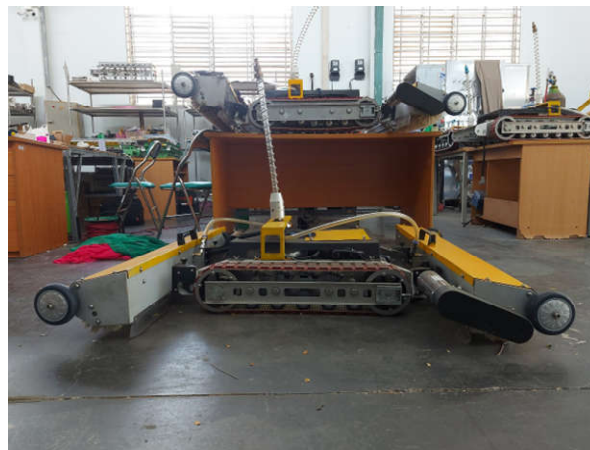
Figure 12. Solar panel cleaning robot, experimental body module
