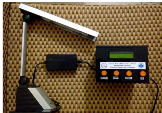
Fig. 112. UVB 311 nm narrow-band medical lamp system.
