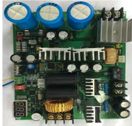
Fig. 75. The PCB main board after soldering all components
