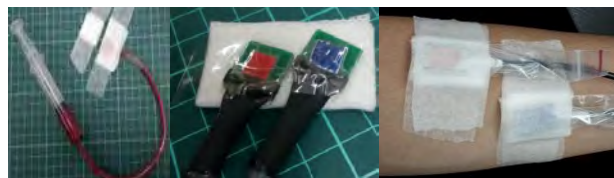
Fig. 4. The stability test: Blood emulation kit, static test, and dynamic test.
