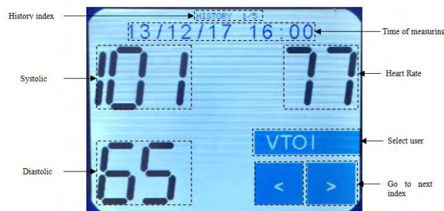
Fig. 58. The LCD with 320x240 in Tele-Blood Pressure
