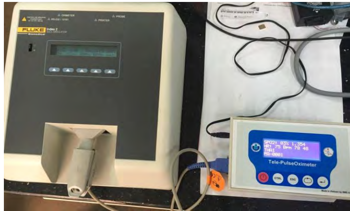
Fig. 36. Calibrated the Spo2 device with Simulator Fluke Index 2
