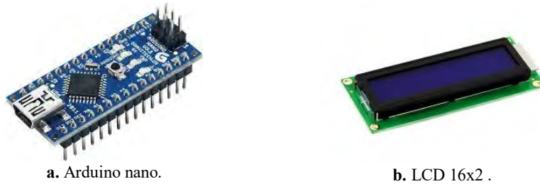
Fig. 2. Arduino nano [9] and LCD 16x2 [8].
