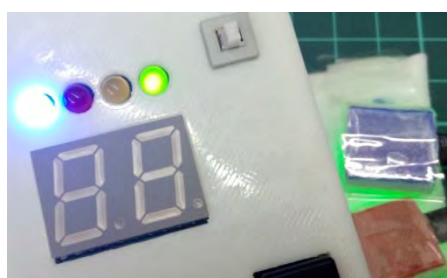
Fig. 8. The blue LED lights up when venous site blood leaking is detected.
