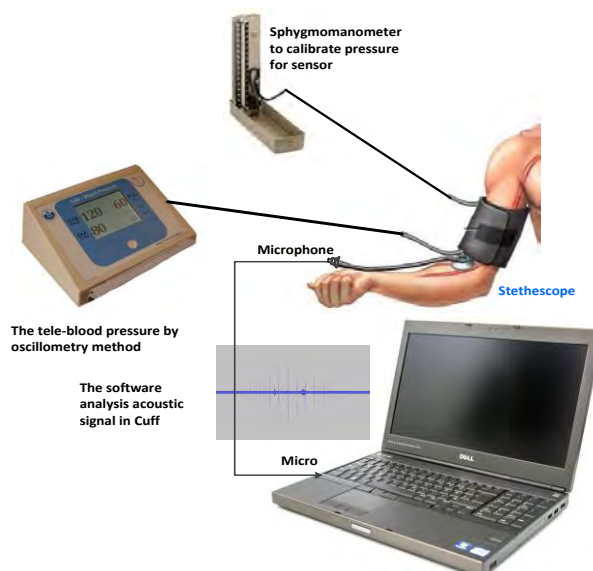
Fig. 60. The method of calibration between sphygmomanometer and our devices.
