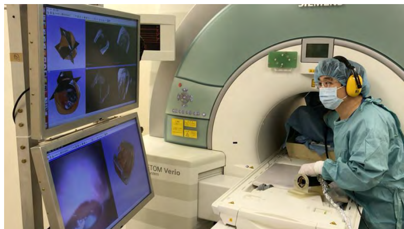
Fig. 3. Experimental setup and trials using the developed MR-compatible endoscope, the navigation software displayed on the MR-compatible in-room monitors, and a 3T MRI scanner.
