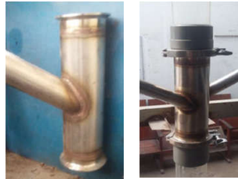
One circular inlet (I.D 38mm)
