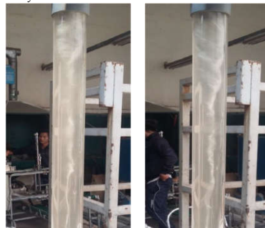
(a) Excavated vortex flow ( V_{sl}=0.27 m/s, V_{sg}=10.5 m/s) (b) Deeply excavated vortex flow ( V_{sl}=0.41 m/s, V_{sg}=6.4 m/s)
