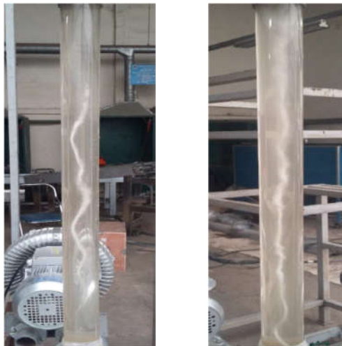
One circular inlet Two circular inlets Figure 9. The filament core in the GLCC lower part
