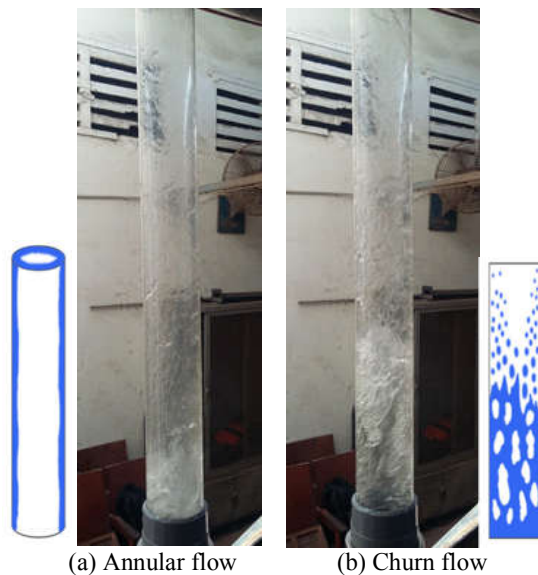
Figure 6. Schematics of different LCO flow regimes ( V_{sl} = 0.341 m/s; V_{sg} = 7.583 m/s)
