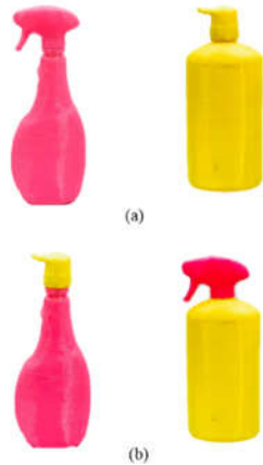
Fig. 7 Results of additive manufacturing for the first example, (a) before cap exchange, and (b) after cap exchange.
