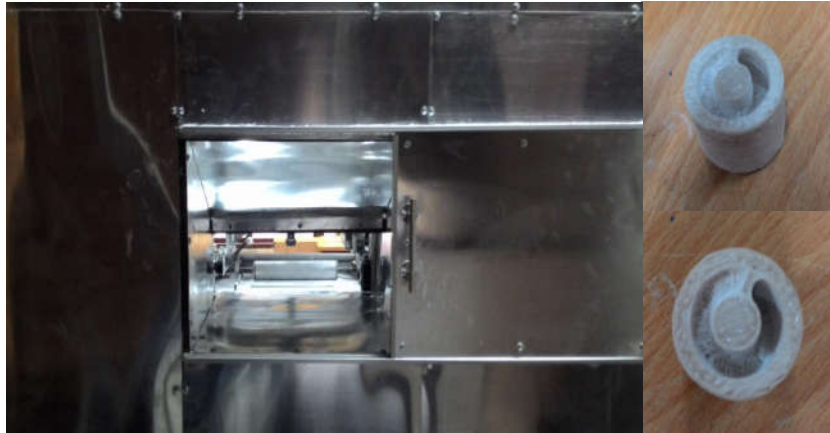
Figure 36. Experiment and molding products by SLS rapid prototyping machine
