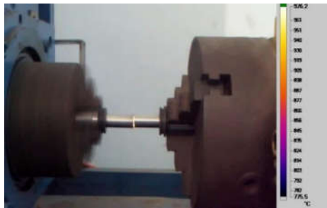
b) Surface temperature distribution along the interface obtained by infrared thermography
