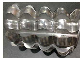
Fig. 15 Hob for cycloid discs [4]
