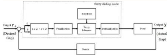
Fig. 8 Scheme of the Fuzzy-Sliding mode controller.
