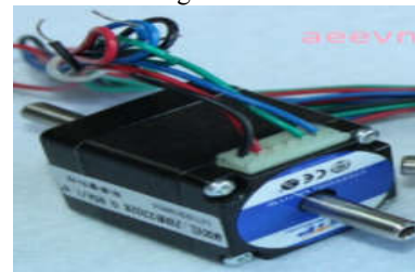
Figure 6: A 2 shafts Gear DC motor for pump [2]
