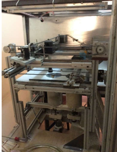
Figure 29. Total manufactured and assembled lifting carriage module
