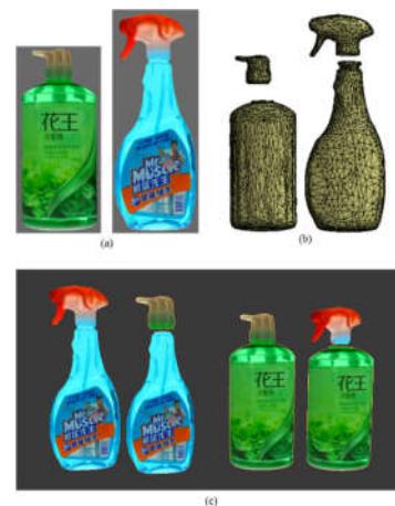
Fig. 6 Design modification using 3D color models, (a) two 3D color models, (b) parts separation with the help of the texture, and (c) parts exchange in the texture mode.
