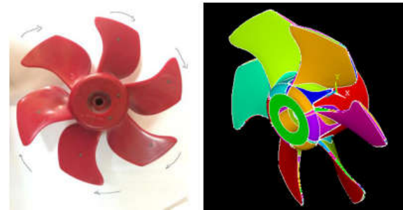
Figure 7. Result of the 3D scan of the propeller
