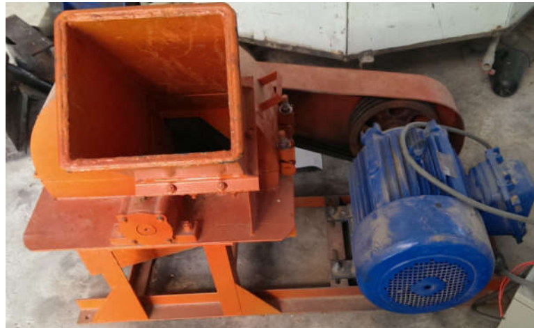
Figure 5. Experimental bamboo grinding machine
