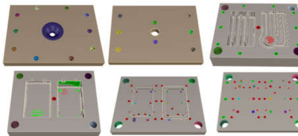
Fig. 7: Results of hole recognition for the mold base in Fig. 1.
