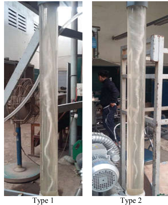
Figure 9. The filament core in the GLCC lower part
