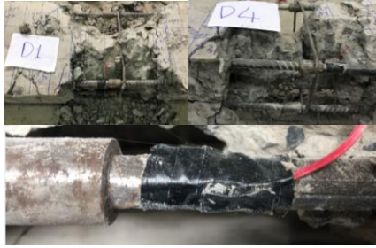
Fig. 8. The coupler of D1 and D4 beam after beams destroyed
