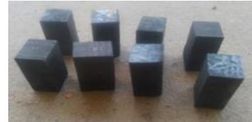
c) SKD61 steel samples after annealing
