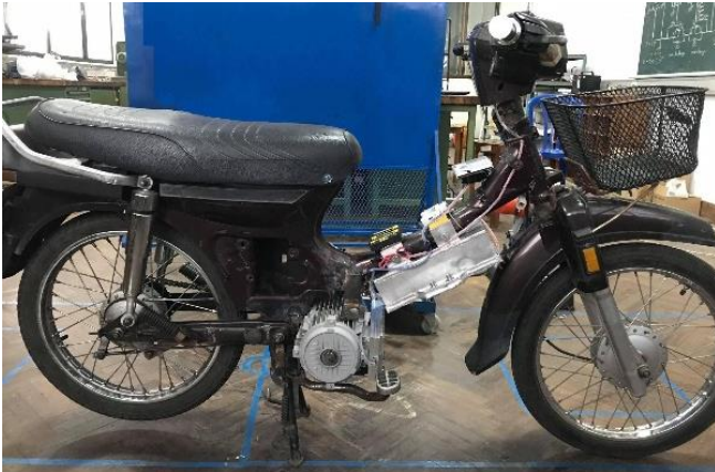
Fig. 11. The induction motor applied in electric motorcycle model.
