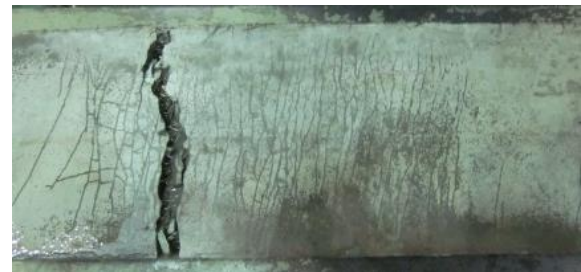
c) Big flexural specimen, crack spacing=4.69 mm
