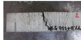
a) Small flexural specimen, crack spacing=3.85 mm
