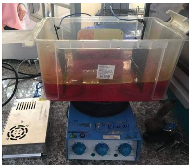
Fig. 1. Experimental set-up for electro-Fenton treatment of dye wastewater
