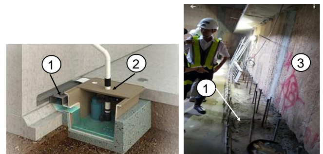
Fig. 1. (a) A schematic of basement-drainage system. (b) a drainage system on construction drain. 1: channel drain (ditch), 2: water pump, 3: Barrette wall
