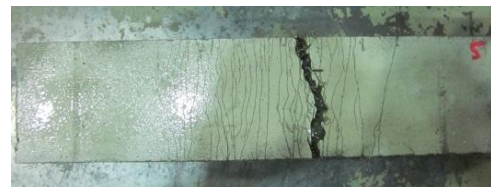
b) Medium flexural specimen, crack spacing=4.55 mm
