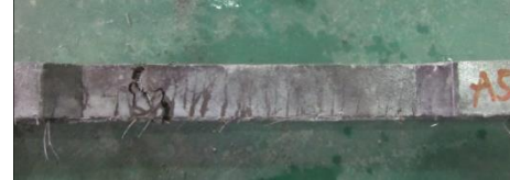
a) Small tensile specimen, crack spacing=6.41 mm
