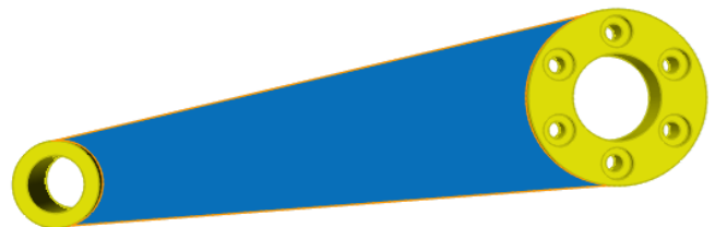
Fig. 3. Geometric model of the upper arm.
