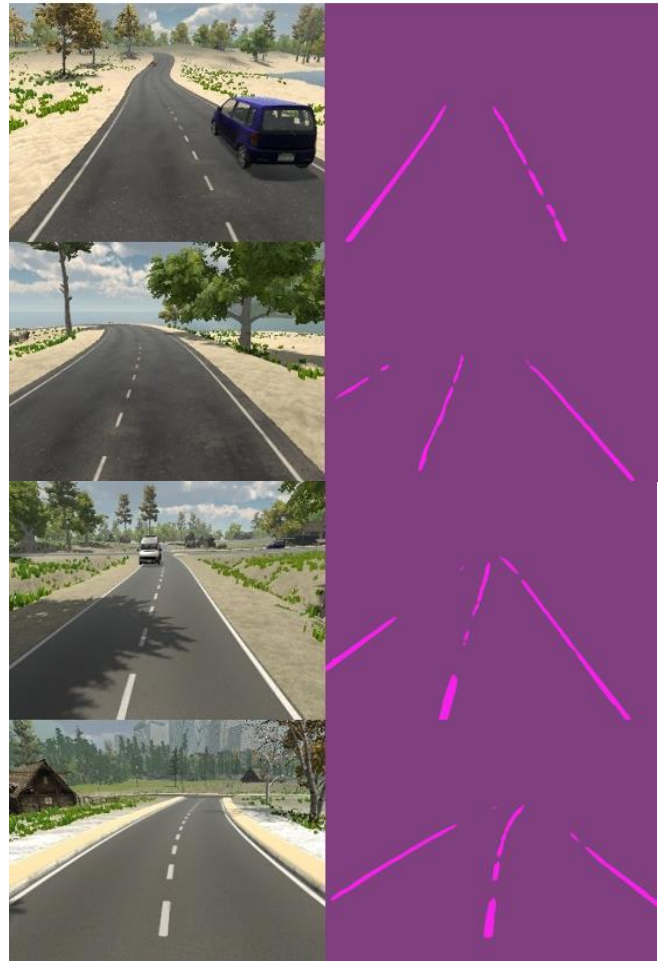
Fig 9. Lane segmentation results on the simulated environment
