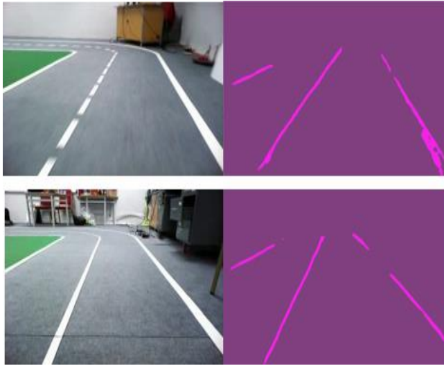
Fig 10. Lane segmentation results on small driving environment.
