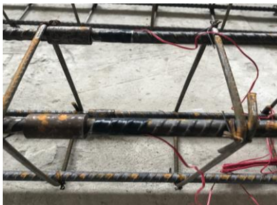
Fig. 3. Strain gauges attached to the steel reinforcement
