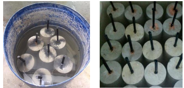
a) Normal water immersion b) Sea water immersion
