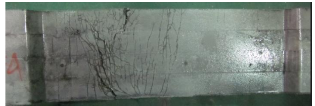
b) Big tensile specimen, crack spacing=13.30 mm
