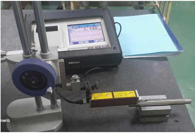
Fig. 2. Surface roughness measuring instrument (Mitutoyo).
