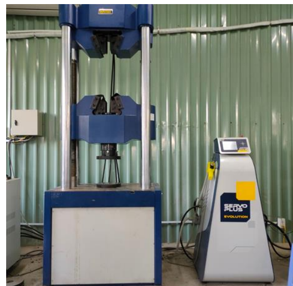
Figure 3. Tensile/compression machine and Servo-plus evolution touch screen system
