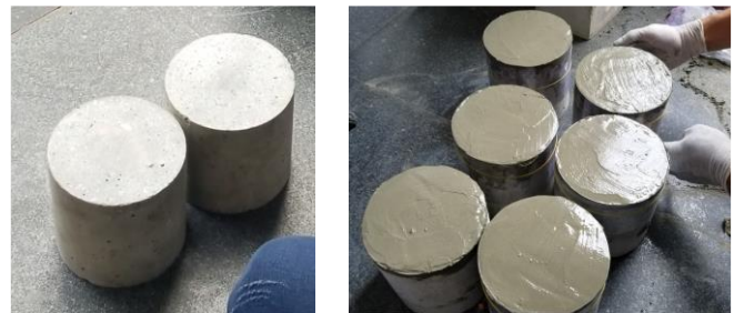
Fig. 6. Samples without waterproofing layer (left), Samples with waterproofing layer (right).
