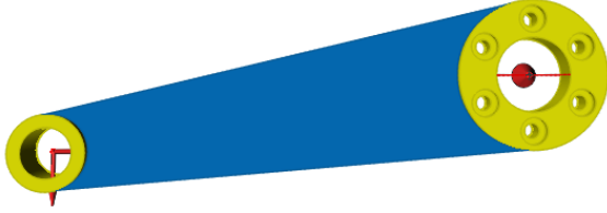
Fig. 7. Model of design space, support and forces.
