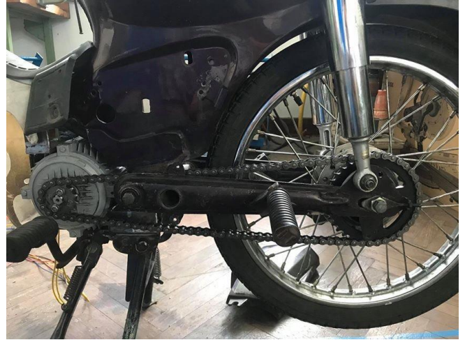
Fig. 12. The powertrain of electric motorcycle model.
