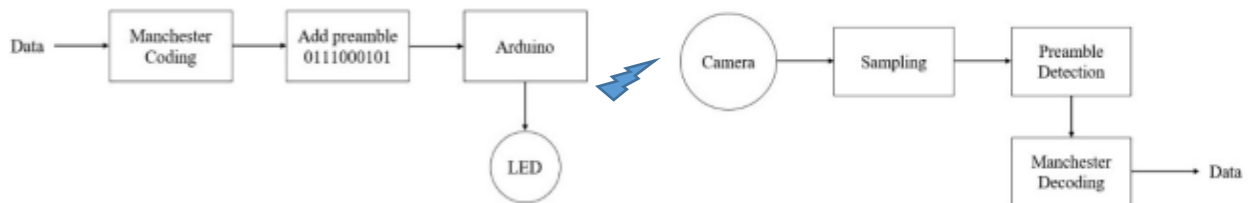
Figure 3. Diagram of Tx pulse modulation (left) and Rx decoding (right)
