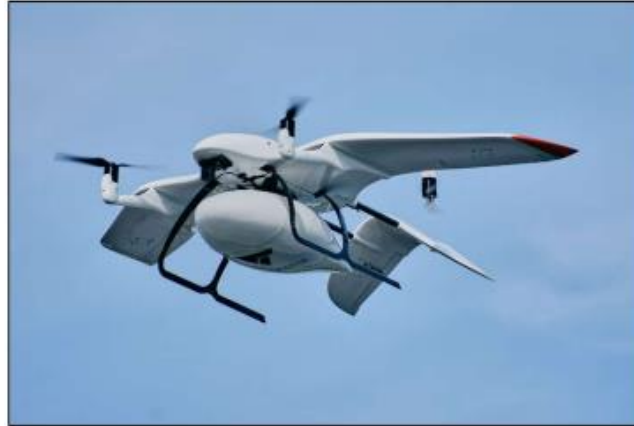
Figure 2. Wingcopter HL178 in copter mode with removable cargo box
