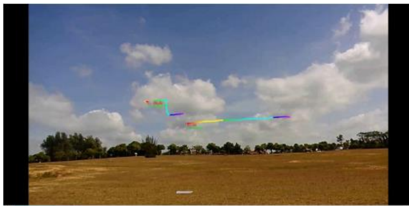
Fig 11. The snapshot of the KF+KCF combination (K-KCF) tracking result from the video footage at 00:15
