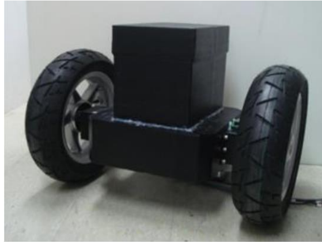
Figure 1. Configuration of two-wheeled MIP platform
