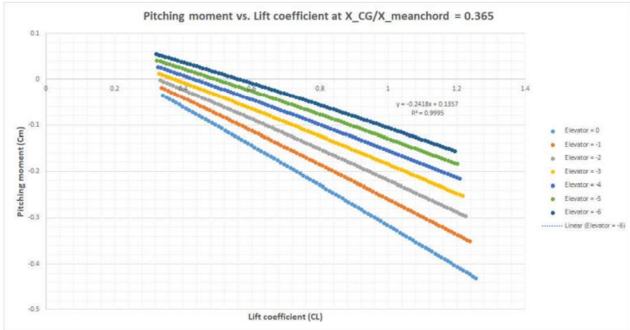
Figure 12. The pitching moment characteristic according to the angle set by the elevator at the center of gravity
