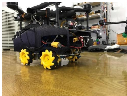
Figure 6: Jetbot implemented with P-DroNet onboard Jetson Nano
