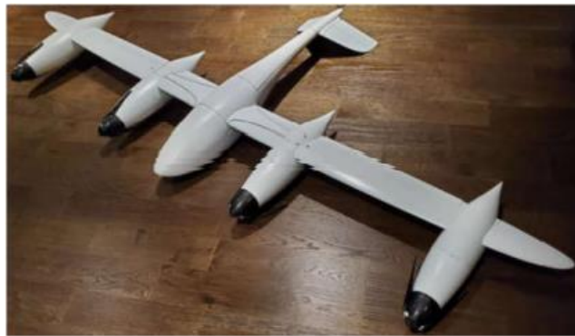
Figure 1. A design of HSUAV for wild area aerial protective inspector
