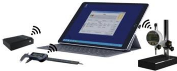
Fig .25 Measuring system according to the IOT protocol
