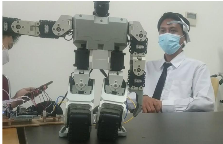
Figure 6. The subject sees and imagines the direction of motion of the robotic arm
