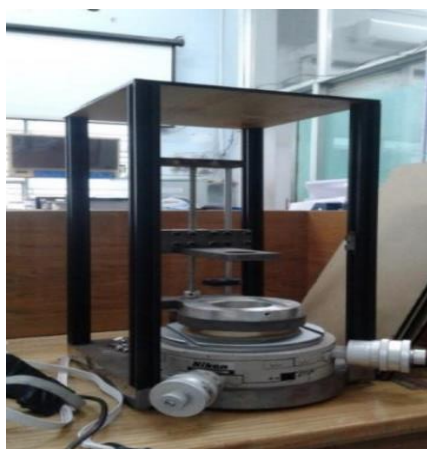
Fig. 3. The mini photolithography device at BiSAE lab (VNUHCM - University of Science, VNUHCM) for the mask aligner.
