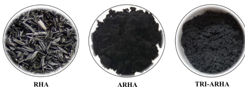
Figure 1. Raw rice husk ash (RHA), activated rice husk ash (ARHA) and activated rice husk ash after amine grafting (TRI-ARHA)
