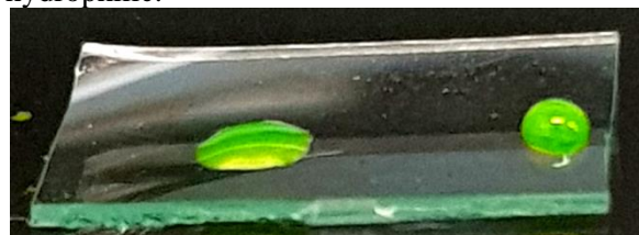
Figure 6. PDMS surface with luminescent solution drops
