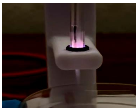
Figure 3. Surface modification of PDMS chip with cold plasma.
