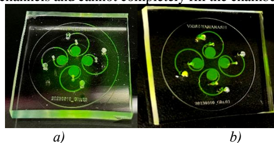
Figure 7. Solution filled into the chambers of the chip a) before and b) after denaturation with cold plasma.
