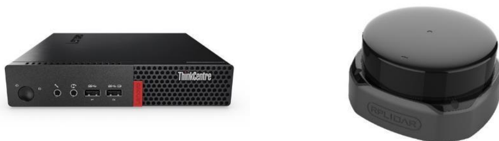
Figure 6. Central controller (Mini PC ThinkCentrer M75q) 1 and Rplidar Laser Sensor S2 2
