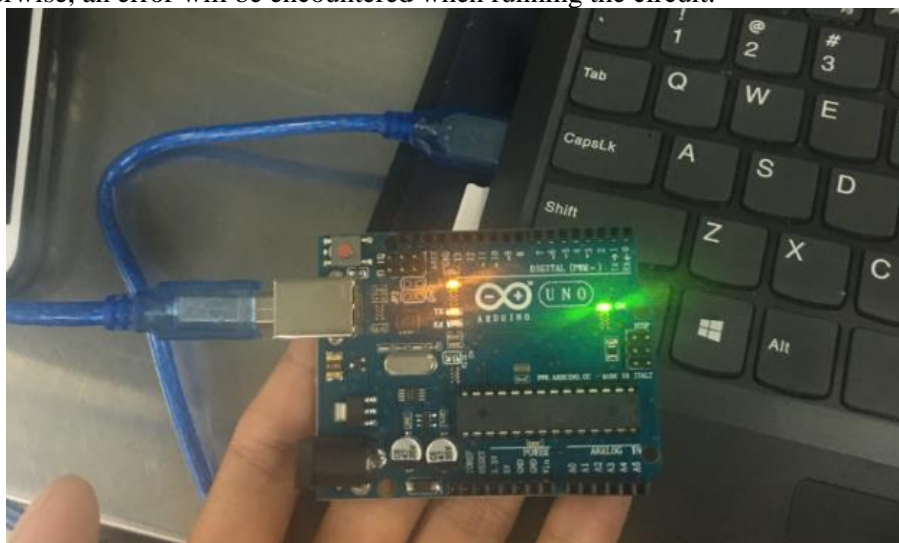
Figure 2: Connect the USB port of the Arduino circuit to the computer.
