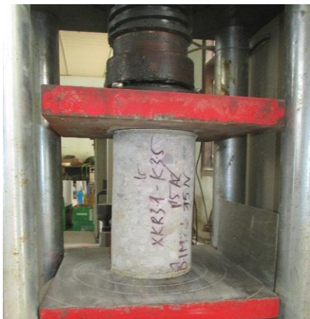
Figure 4: Compression test on the specimens.
