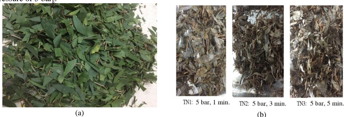
Figure 5: Quinquenervia materials after steam explosion at 3 different holding durations.
