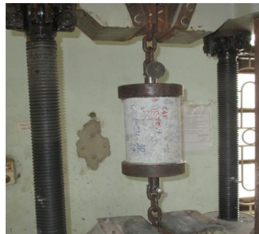
Figure 5: Tensile test on the specimens.
