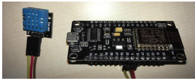
Figure 2. ESP8266 with DHT11
