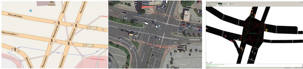
Figure 4. Intersection Geometry from left to right: Complex traffic light controlled intersection, satellite view of complex intersection and SUMO traffic simulation with junction connections shown.
